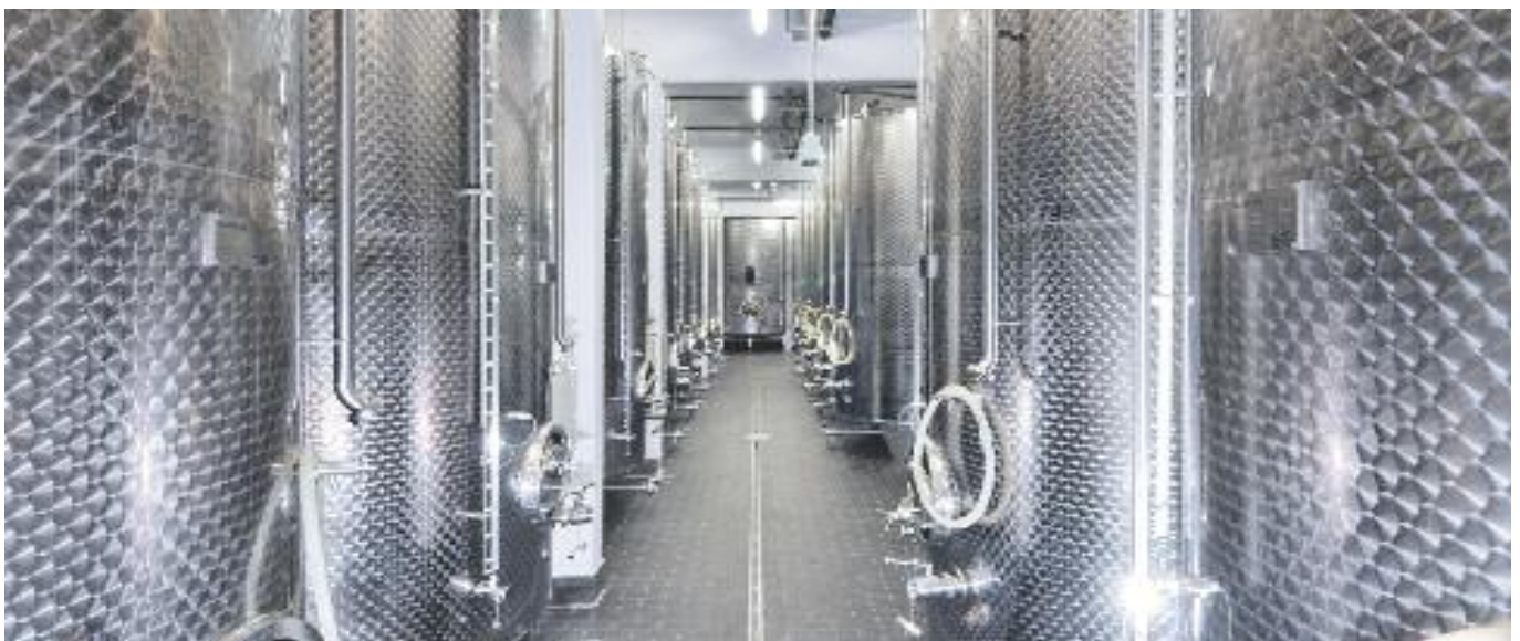
Computer- and temperature-controlled stainless steel tanks
